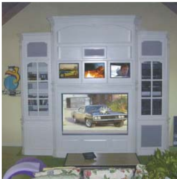
Figure 12. A family room theater is a step up from a theater in a box because all the elements are built in. In this theater, the front speakers and screen are fully housed in a cabinet. The woofer is at bottom right and the rear speakers are built into the wall.
