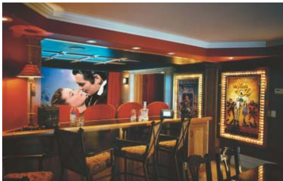
Figure 2. Pilasters, soffits, and ceiling trims not only look good, but also enhance audio reproduction in a theater by breaking up large flat surfaces.
