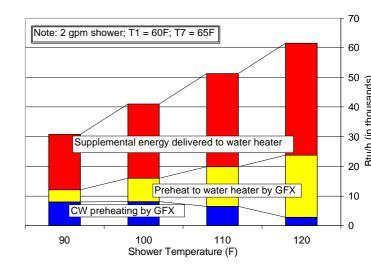
showers (e.g. 120°F), most of the energy from the GFX is used for preheating hot water. Over the range of shower temperatures studied, the GFX saved about 40% of the total energy needed for the shower in this experiment.
