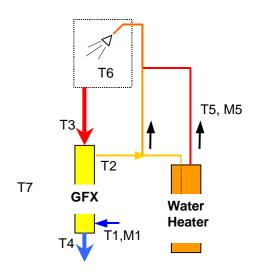
We found that the GFX could raise temperature of the inlet temperature from 60°F to 85°F by maintaining shower conditions at 2.0 GPM and 120°F (water heater setpoint). We noticed that under these conditions, the temperature of the wastewater inlet to the GFX unit (T3) was 12 F° lower than
