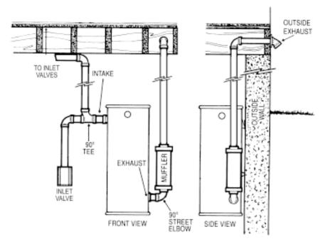
enclose. If the unit is to be located in a closet or utility room it must be vented. Louvered doors fulfill this purpose. A muffler can, of course be used to minimize noise.
