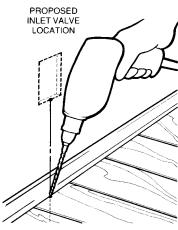
the proposed location. Holding the drill vertical and as close to the wall as possible drill a small pilot hole through the floor and sub floor. The straight section of a wire coat hanger cut at an angle makes a good pilot hole drill bit. (Be careful not to snag carpeting.)
