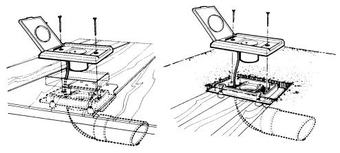
floor. In the case of linoleum or uncovered floors the mounting plate will be installed from below. If the floor is carpeted cut a hole in the carpet with a utility knife and slip the <u>untrimmed mounting plate</u> under the carpet. Fasten the mounting plate to the floor with screws. A coupling and a short piece of tubing may be required as a spacer between the mounting plate and the 90 degree fitting below.
