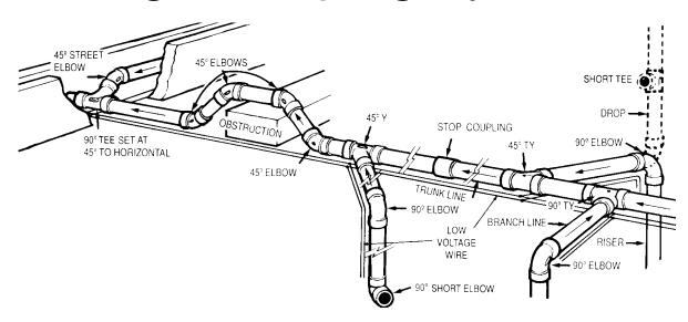
The amount of airflow that reaches the hose is dependent on the efficiency of the layout of the tubing system. Lines are to be kept as straight as possible. Tight 90 degree fillings are to be used only at inlet valve locations and sweep 90's used in all other applications.
