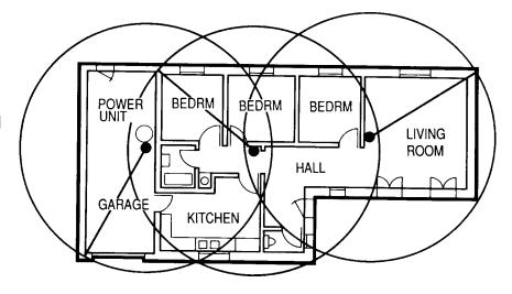
string or the hose itself can be used to help plan the layout. If working with 1/4" scale blueprints a seven-inch string can be used to represent the hose. If an electrical beater brush is to be used at present or in the future the inlet valve should be located within five feet of an electrical outlet. Air-turbine driven beater brush heads do not require electricity and thus allow more flexibility when choosing inlet valve locations.
