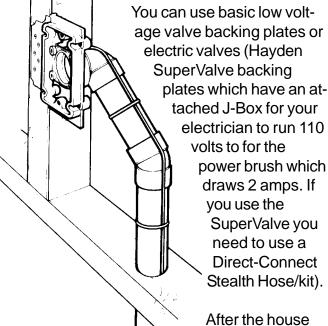
has been wired and plumbed, but before the dry wall is installed is the best time to pipe in a central vacuum tubing system. Locate the inlet valve locations and nail the mount-
